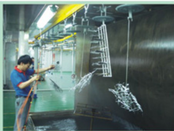
手動噴鍍懸掛綫 manual spray plating suspension line
